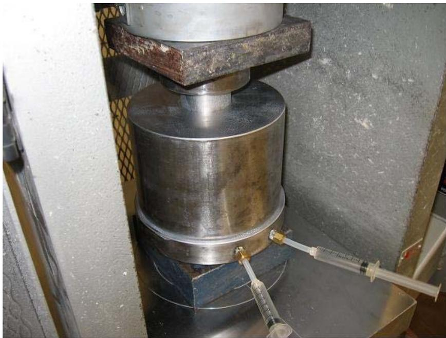
FIGURE 4. DIE ASSEMBLY WITH ATTACHED POLE FLUID COLLECTION SYRINGES.
