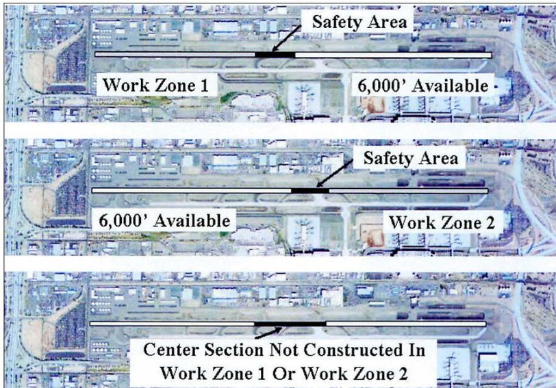
Figure 2-1. Illustration of Phoenix phasing.
