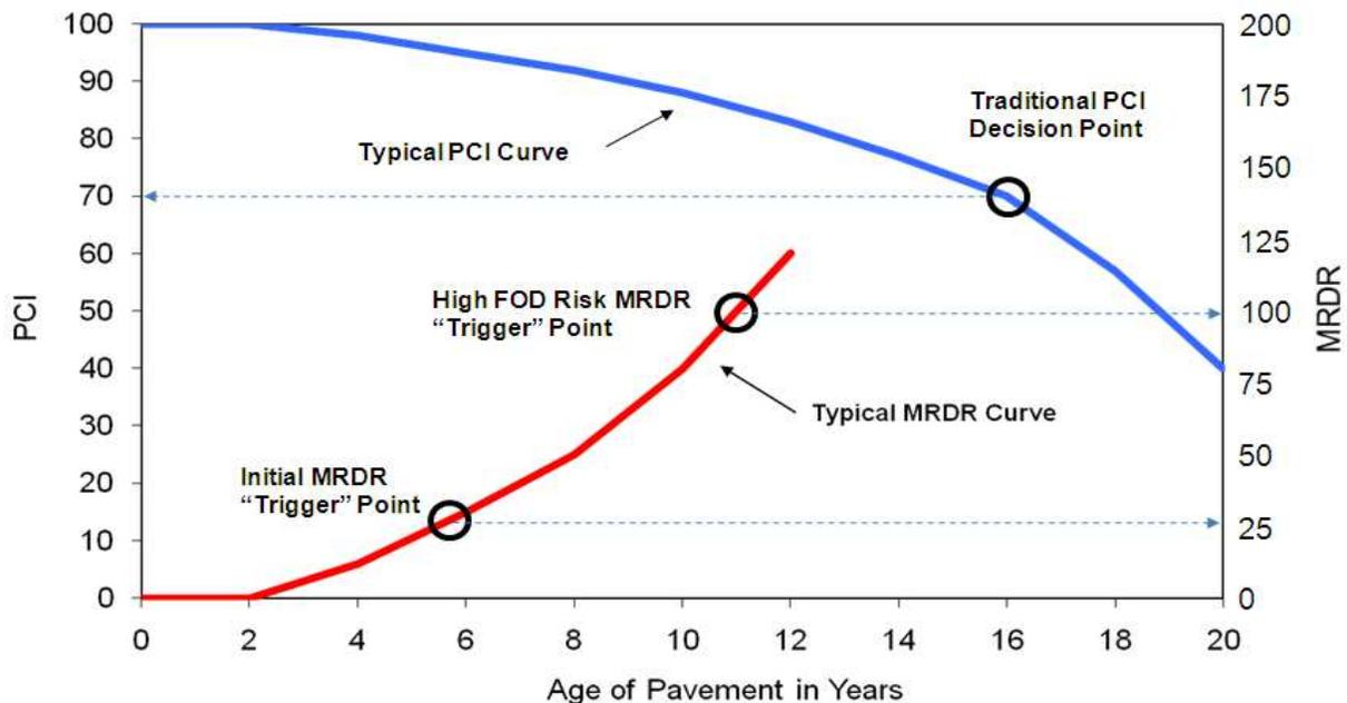
Figure 21. Illustration of trigger points for PCI and MRDR.
