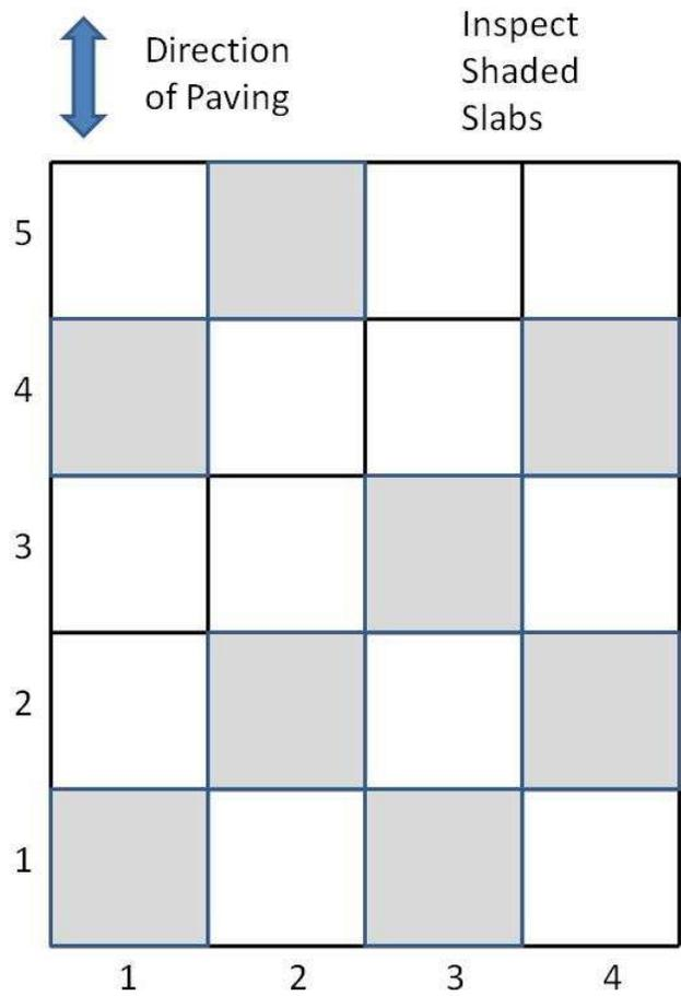
Figure 2. Recommended slab locations for a network-level inspection in a typical 20-slab sample unit.
