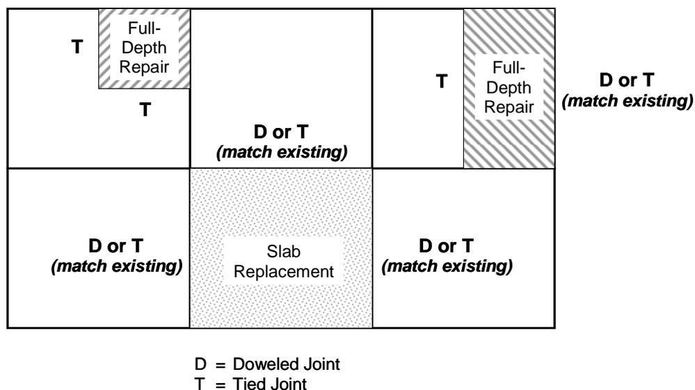
Figure 25. General jointing schematic for full-depth repairs on airfield pavements.
