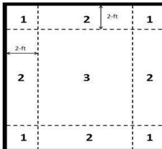
Figure 3. Typical slab layout showing the three locations (1: corner, 2: joint, and 3: interior).
