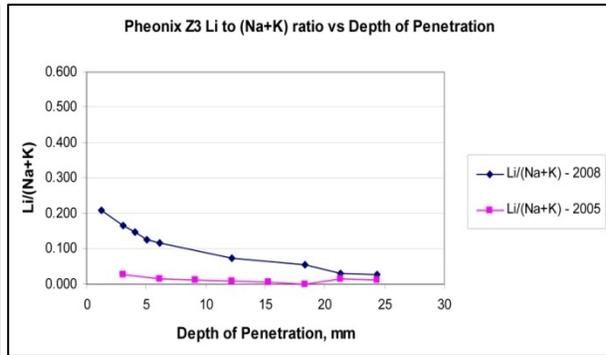
**Figure 34: Graph Results Phoenix Multiple Application - Lithium to Alkali Equivalent Ratio vs. Depth of Penetration 2005 & 2008**
