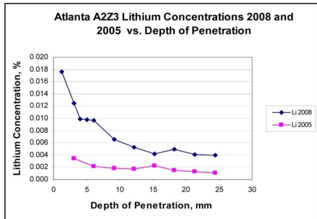
**Figure 41: Graph Results Atlanta Area 2 Multiple Applications - Lithium Concentration vs. Depth of Penetration 2005 & 2008**
