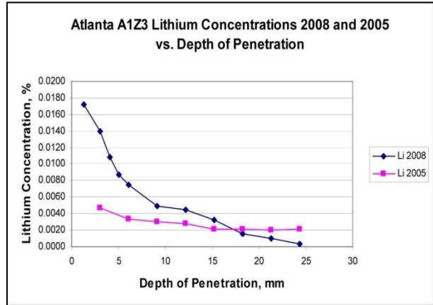
**Figure 39: Graph Results Atlanta Area 1 Multiple Applications - Lithium Concentration vs. Depth of Penetration 2005 & 2008**
