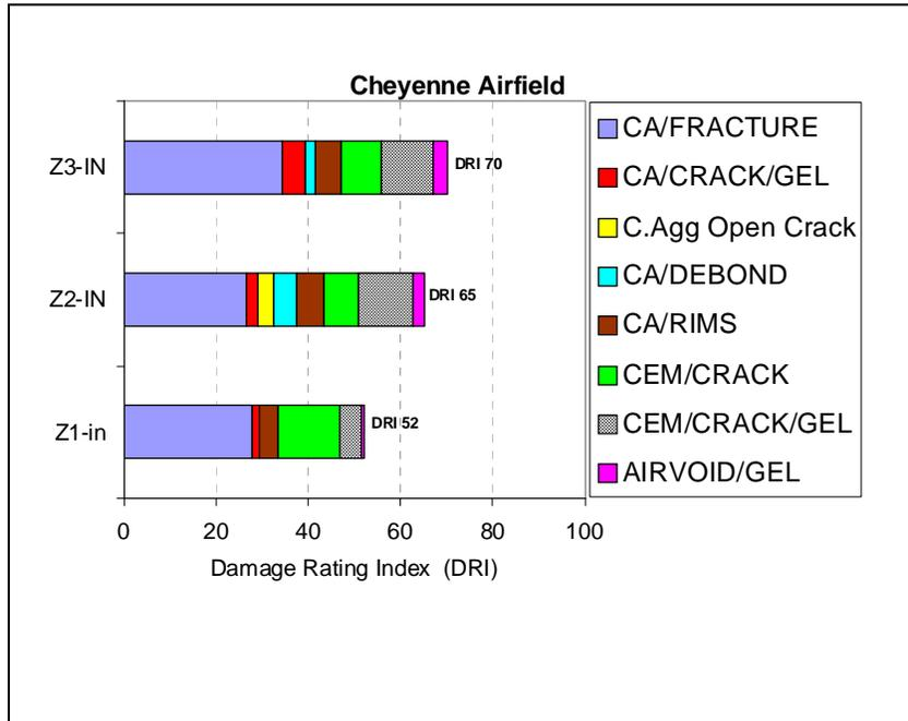
**Figure 23: Chart showing Damage Rating Index (DRI) of cores from Cheyenne Regional Airport**
