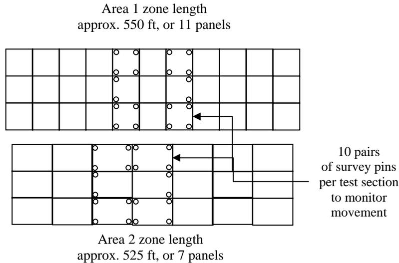
**Figure 12: Schematic of Survey Point Layout at Hartsfield-Jackson Atlanta International Airport**
