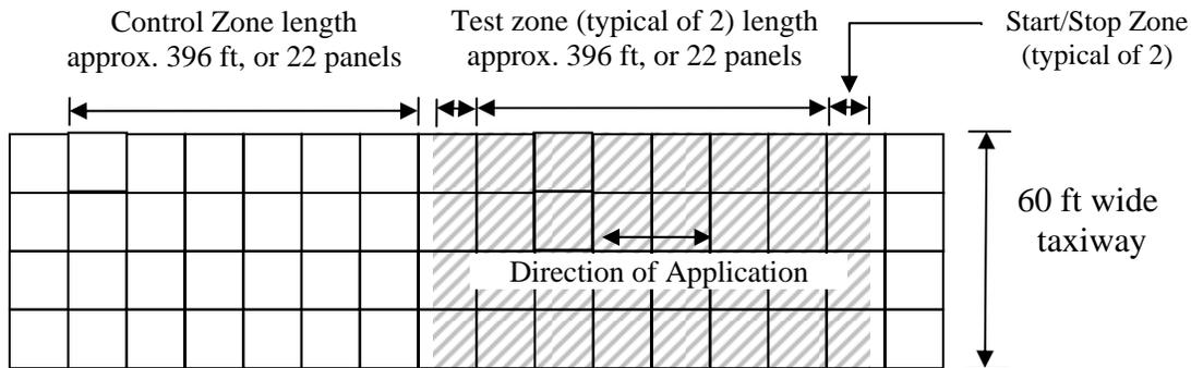
**Figure 2: Schematic of Test and Control Zones on Taxiway Bravo at Cheyenne Regional Airport**
