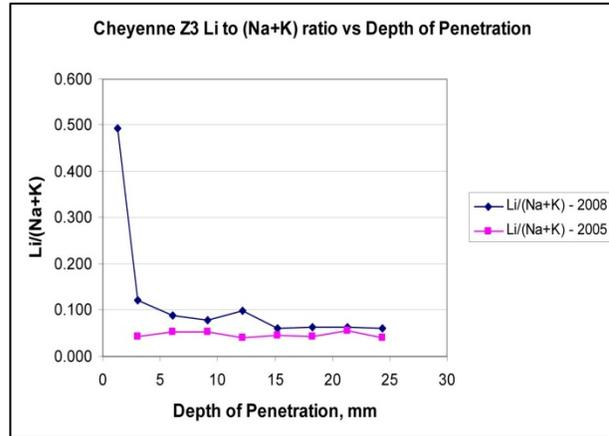
**Figure 28: Graph Results Cheyenne Multiple Applications - Lithium to Alkali Equivalent Ratio vs. Depth of Penetration 2005 & 2008**
