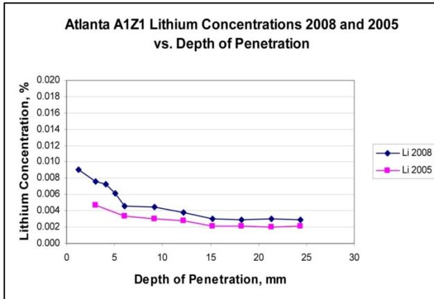
**Figure 38: Graph Results Atlanta Area 1 Single Application - Lithium Concentration vs. Depth of Penetration 2005 & 2008**
