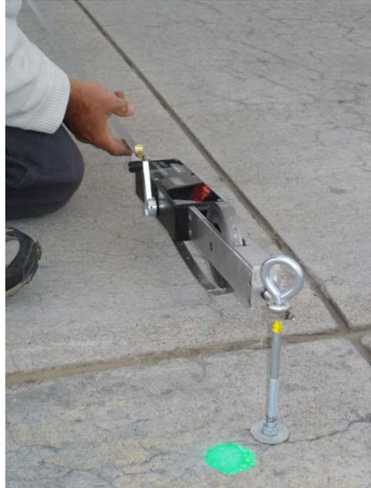
**Figure 8: Extensometer Measurement at Cheyenne Regional Airport**
