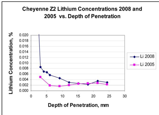
**Figure 25: Graph Results Cheyenne Single Application - Lithium Concentration vs. Depth of Penetration 2005 & 2008**
