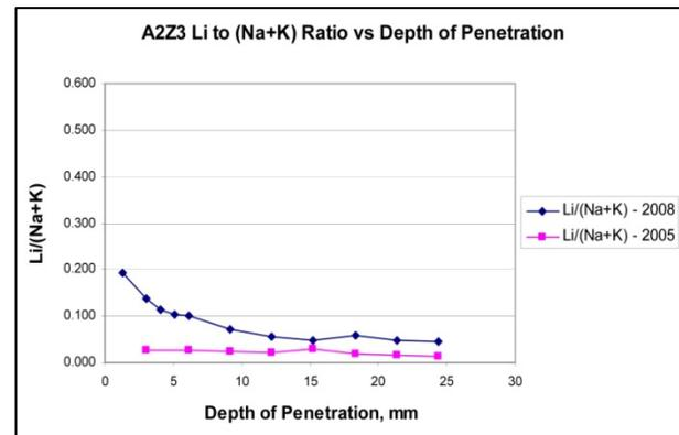
**Figure 45: Graph Results Atlanta Area 2 Multiple Applications - Lithium to Alkali Equivalent Ratio vs. Depth of Penetration 2005 & 2008**
