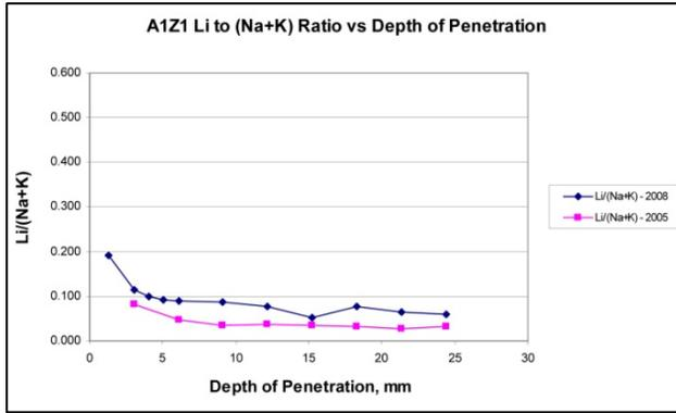
**Figure 42: Graph Results Atlanta Area 1 Single Application - Lithium to Alkali Equivalent Ratio vs. Depth of Penetration 2005 & 2008**
