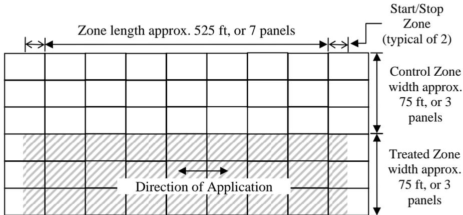
**Figure 7: Schematic of Area 2 Control and Test Zone (Typical of 2) Layout at Hartsfield-Jackson Atlanta International Airport**
