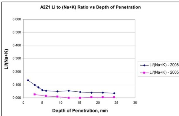
**Figure 44: Graph Results Atlanta Area 2 Single Application - Lithium to Alkali Equivalent Ratio vs. Depth of Penetration 2005 & 2008**
