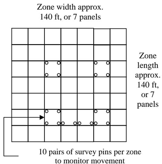
**Figure 11: Schematic of Survey Point Layout at Phoenix Sky Harbor International Airport**
