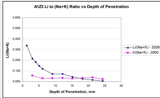
**Figure 43: Graph Results Atlanta Area 1 Multiple Applications - Lithium to Alkali Equivalent Ratio vs. Depth of Penetration 2005 & 2008**
