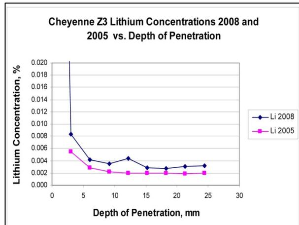
**Figure 26: Graph Results Cheyenne Multiple Applications - Lithium Concentration vs. Depth of Penetration 2005 & 2008**
