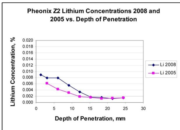
**Figure 31: Graph Results Phoenix Single Application - Lithium Concentration vs. Depth of Penetration 2005 & 2008**
