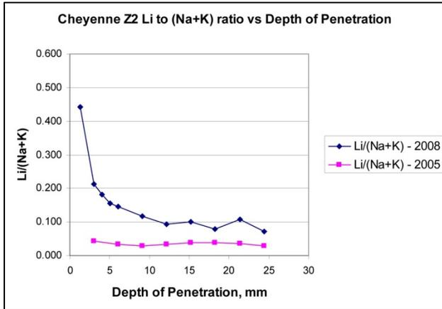
**Figure 27: Graph Results Cheyenne Single Application - Lithium to Alkali Equivalent Ratio vs. Depth of Penetration 2005 & 2008**
