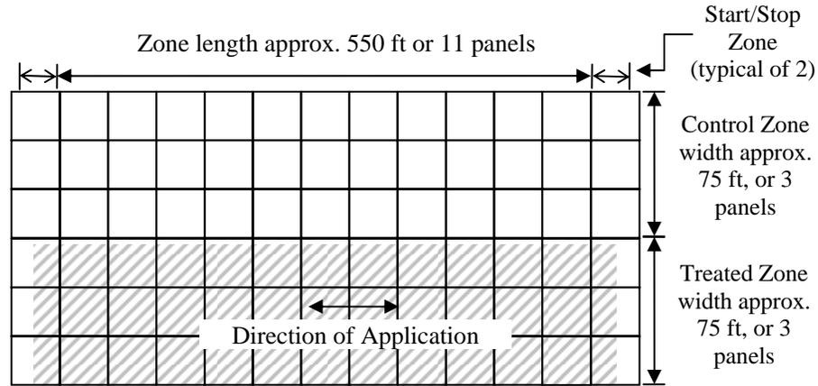
**Figure 6: Schematic of Area 1 Control and Test Zone (Typical of 2) Layout at Hartsfield-Jackson Atlanta International Airport**
