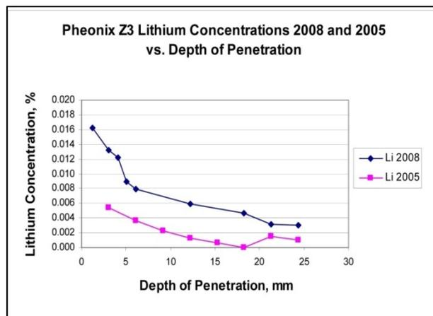
**Figure 32: Graph Results Phoenix Multiple Applications Lithium Concentration vs. Depth of Penetration 2005 & 2008**
