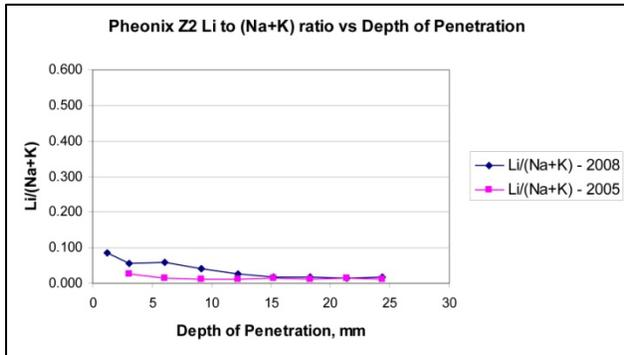
**Figure 33: Graph Results Phoenix Single Application - Lithium to Alkali Equivalent Ratio vs. Depth of Penetration 2005 & 2008**
