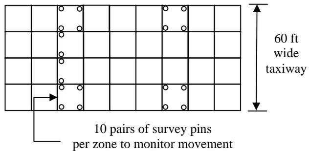
**Figure 10: Schematic of Survey Point Layout at Cheyenne Regional Airport**
