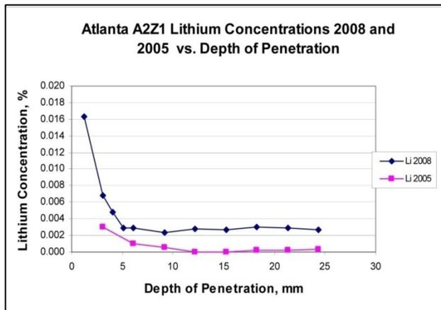
**Figure 40: Graph Results Atlanta Area 2 Single Application - Lithium Concentration vs. Depth of Penetration 2005 & 2008**
