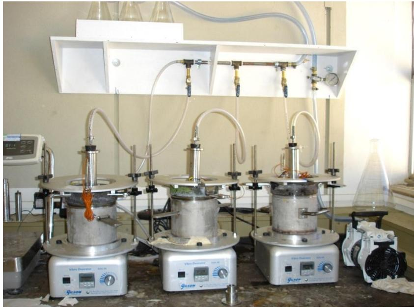
Figure 4-4 Dilatometer vacuuming under vibration.
