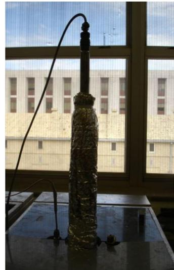
Figure 4-5 (a) Dilatometer placed in water bath after final vacuuming, (b) Dilatometer tower is wrapped with insulating material.
