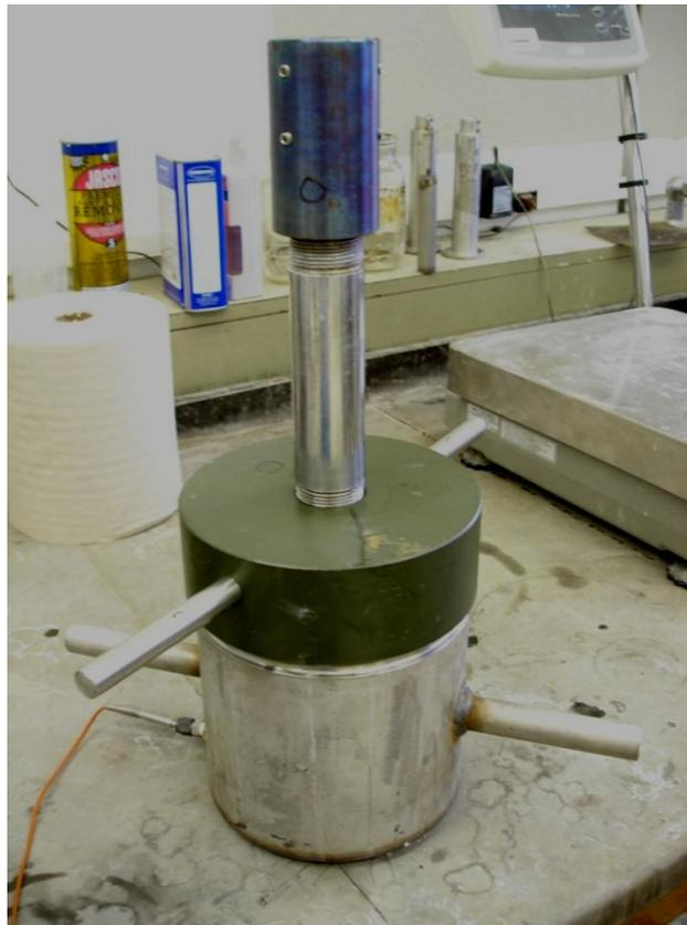
Figure 4-1 Final version of the dilatometer with modified lid and tower.
