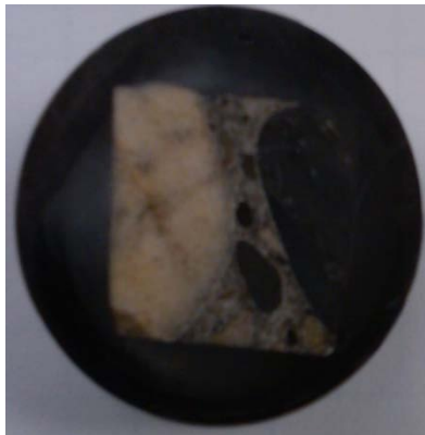
Figure 3. SEM sample prepared for BSE mode and EDS analysis
