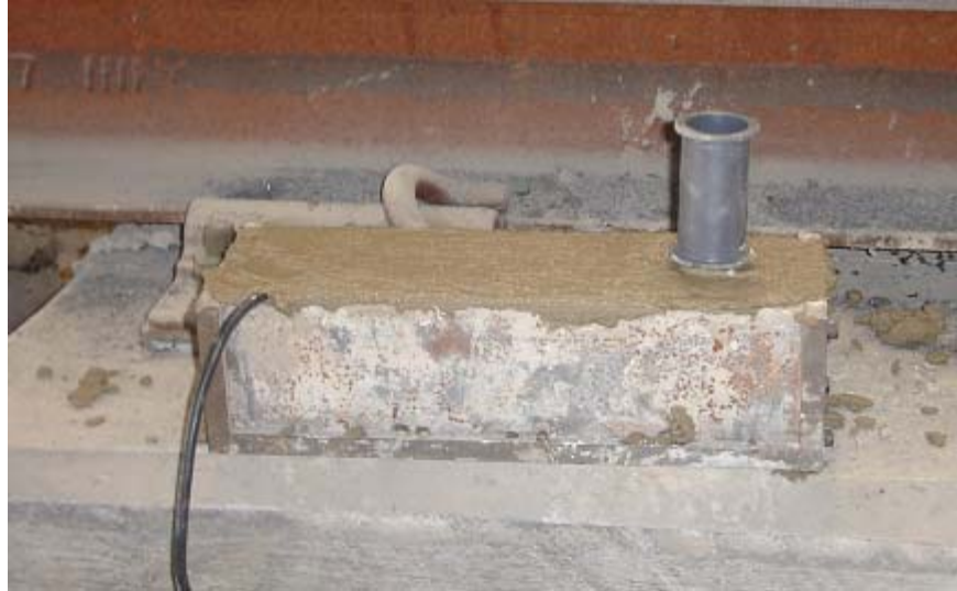
Figure 6 Free Shrinkage Test Setup.
