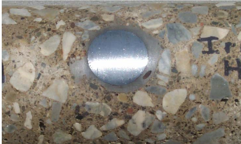
Figure 14a. Core 1 from the control section.
