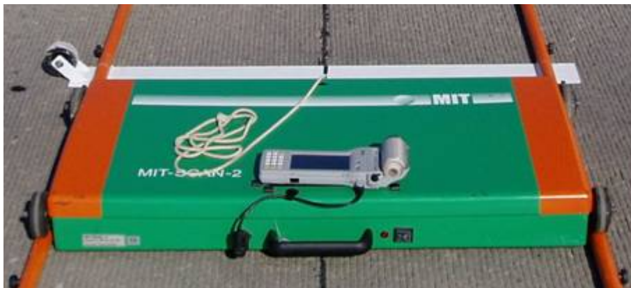
Figure 3. MIT Scan-2, a magnetic imaging device for measuring dowel bar alignment.
